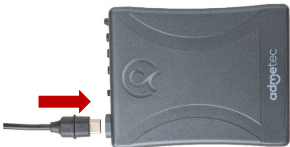
Fig. 03 – Type C cable insert into MCU
